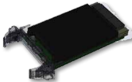
Figure 1 IC-INT-VPX3d equipped with standard air cooled mechanical solution
